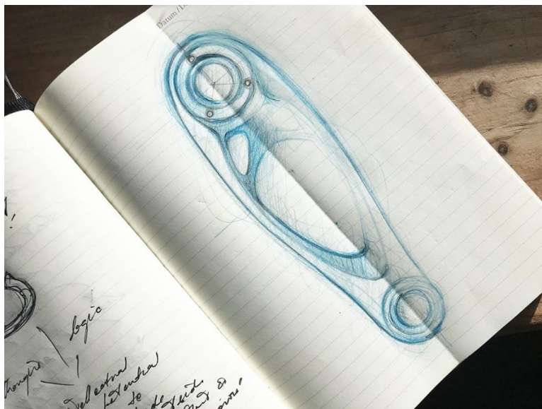
Figure 13. Crank sketch by Roderick Walden, which used the selected topology study as form inspiration. A clear connection with the revised crank design produced by Gianfranco Lassandro (see figure 14) is evident.
